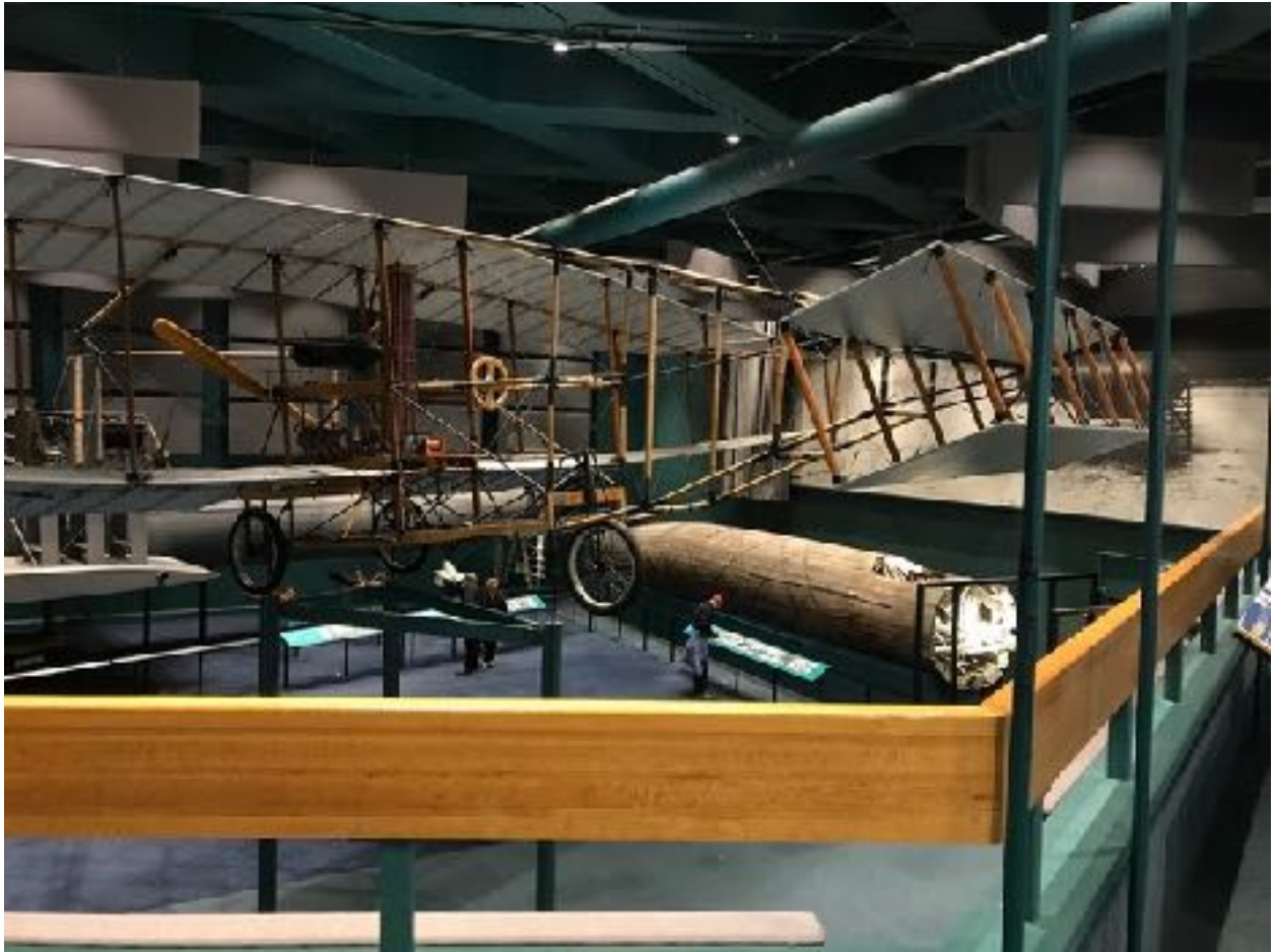
a replica of the Silver Dart, the first powered, heavier-than-air machine to fly in Canada in 1909. The brown, cigar-shaped object on the center right is part of the HD-4 which was the hydrofoil which set the world speed record in 1919.
