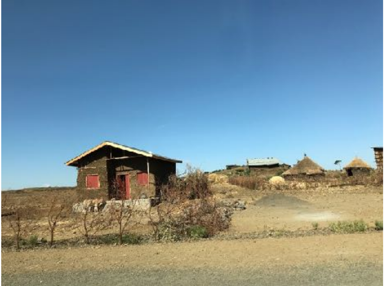
typical house built of sticks with mud/straw to cover the sticks. There is no interior bracing, so it may lean after a while. The round huts were the original houses.
